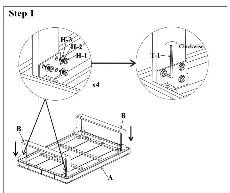
Position Table Top (A) and Legs (B) as shown. Secure using Bolts (H-1), Spring Washers (H-2) and Flat Washers (H-3) with Allen Key (T-1), stacking the hardware in the order as shown. Engage all Bolts (H-1) first before fully tightening.
